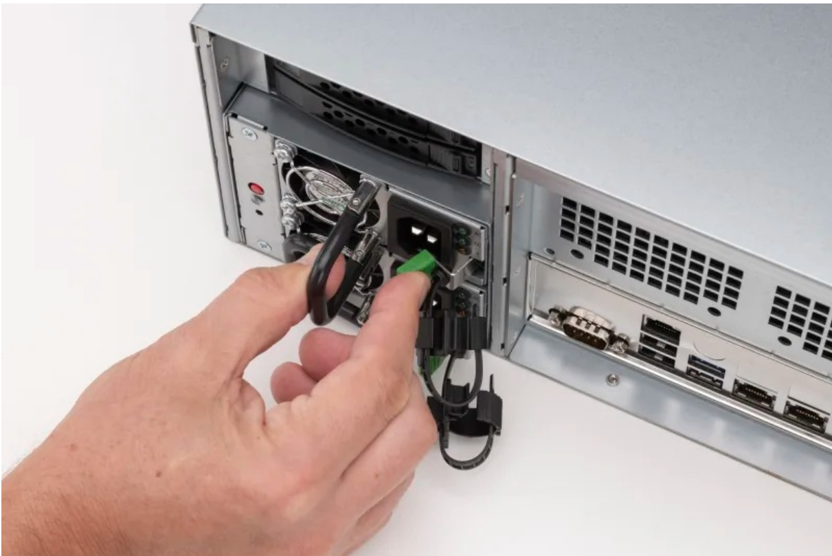
3. Disengage the failed power supply by pulling out while pressing the lever.
